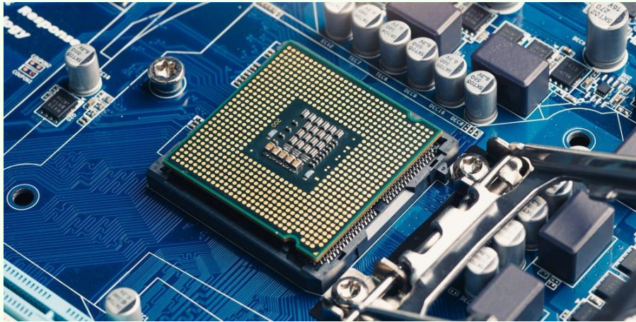
Figure 2 Central Processing unit
